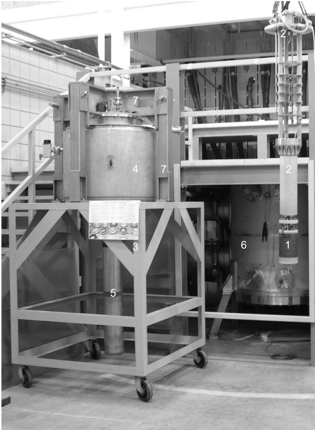
Figure 2-19. View of Cell 4 at the NHMFL. (1) 5T insert, (2) coil support structure hanging from the crane, (3) dewar stand, (4) dewar, (5) dewar tail that fits the bore of the (6) resistive magnet, (7) structure to react fault forces on the insert support structure to the resistive magnet housing.
