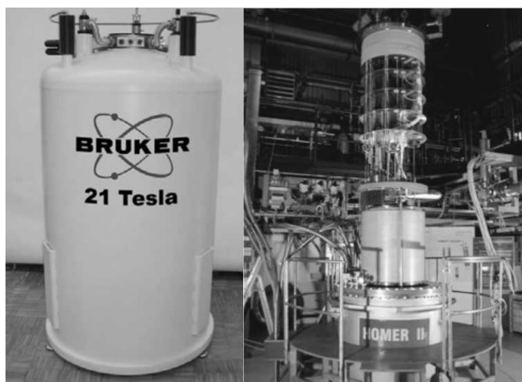
Figure 1-3. (left) Research magnet capable of generating 21 T in a 64 mm cold bore at 2.2 K and 19 T at 4.2K; (right) 20 T research magnet hanging above its 1.4 m diameter cryostat.
