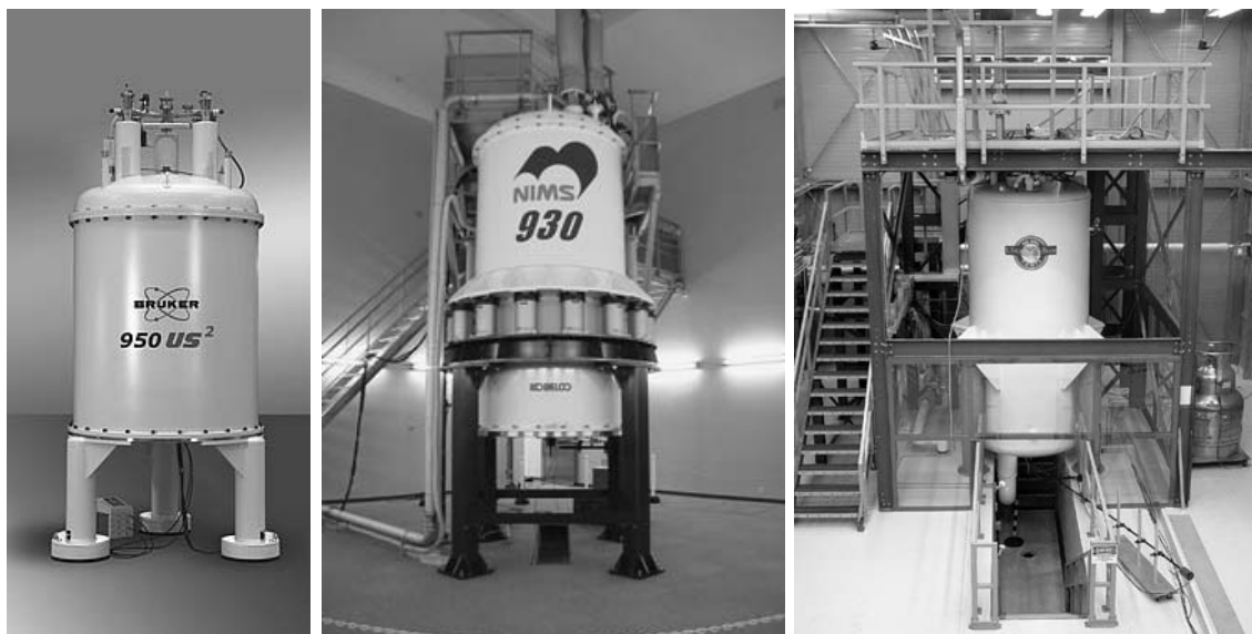
Figure 1-2. (left) A 22.3 T/950 MHz NMR system of 3.3 m radial and 4.6 m axial dimension by Bruker; (middle) the 21.6 T/930 MHz NMR system at the Tsukuba Magnet Lab of NIMS; (right) the NHMFL 21.1 T/900 MHz Ultra Wide Bore NMR system.
